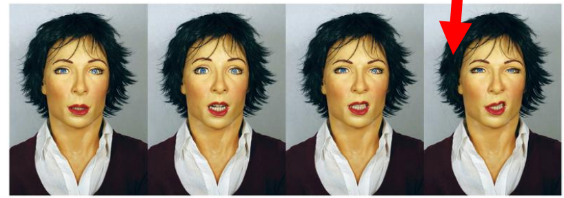
FIGURE 7 | The FACE Robot (Facial Automaton for Conveying Emotions) displaying some of its hyper-realistic facial expressions.
