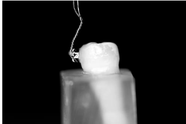
FIGURE 1. Bonded teeth set in acrylic block; a 0.021 \times 0.025 -inch stainless steel wire was ligated into each bracket slot to minimize deformation of bracket during debonding; a 0.020-inch loop was made from 0.012-inch stainless steel ligature wire and placed under the gingival wings of the twin bracket.
